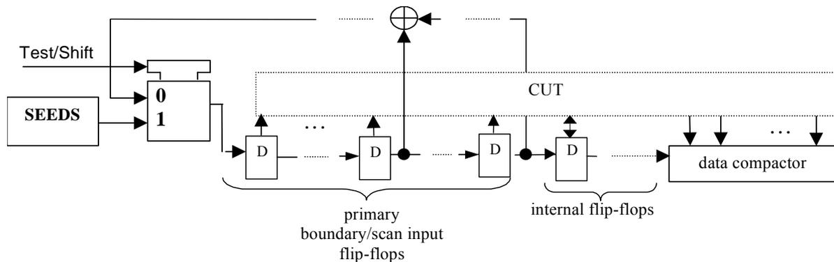
Fig. 1. Proposed mixed mode testing scheme which uses boundary scan with added feedback and partial reseeding of the LFSR
