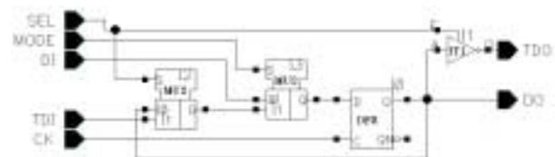
Fig. 10 – Internal sRAS cell
