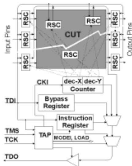
Fig. 2: Modified Random Access Scan – a general scheme
