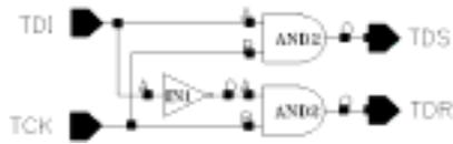
Fig. 3: Set / Reset decoder
