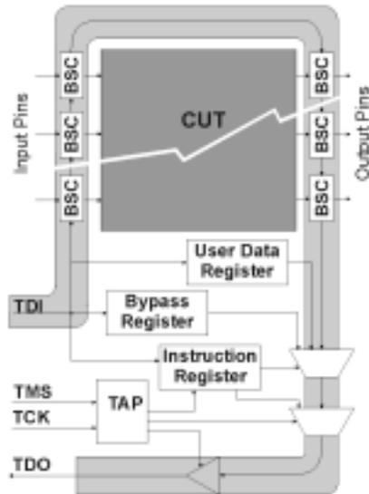
Fig. 1: Boundary Scan – the principle scheme
