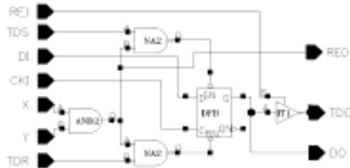
Fig. 4: Proposed internal RAS scan cell
