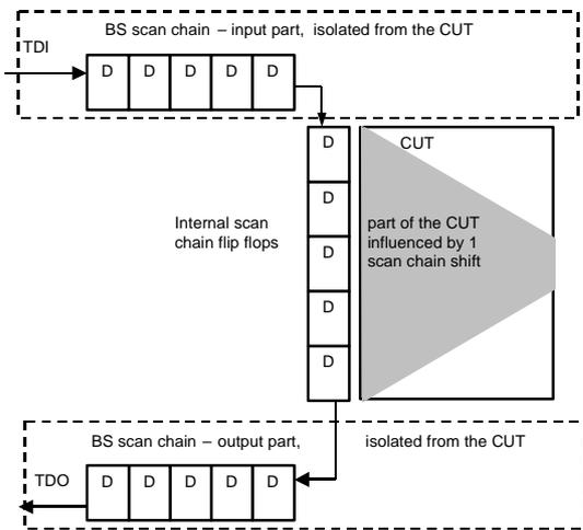
Fig. 1 BS circuit activity during shifting patterns
