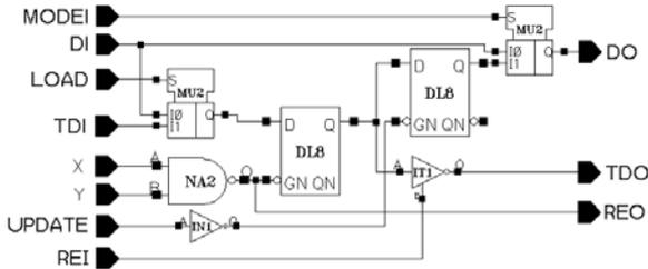
Fig. 6 Proposed I/O RAS scan cell (RSC)
