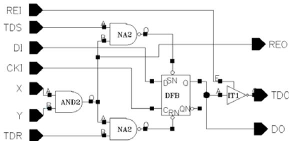
Fig. 4 Proposed internal RAS scan cell
