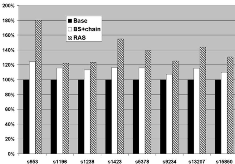
Fig. 7 Hardware overhead (AMS 0.6µm technology) of ISCAS circuits using standard scan chain cells compared with circuits using modified RAS cells.
