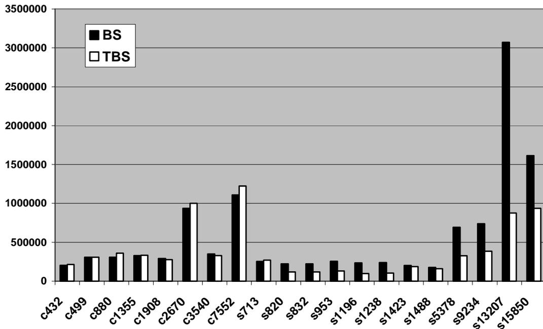
Fig 8: Hardware overhead of the BIST using standard BS and a memory for storing the test patterns compared with the BIST using built-in TPG [ $\mu\text{m}^2$ ] (also Tab. 3.).
