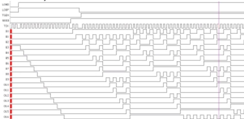
Fig 7: Time diagram of the simulation of the TPG functionality
