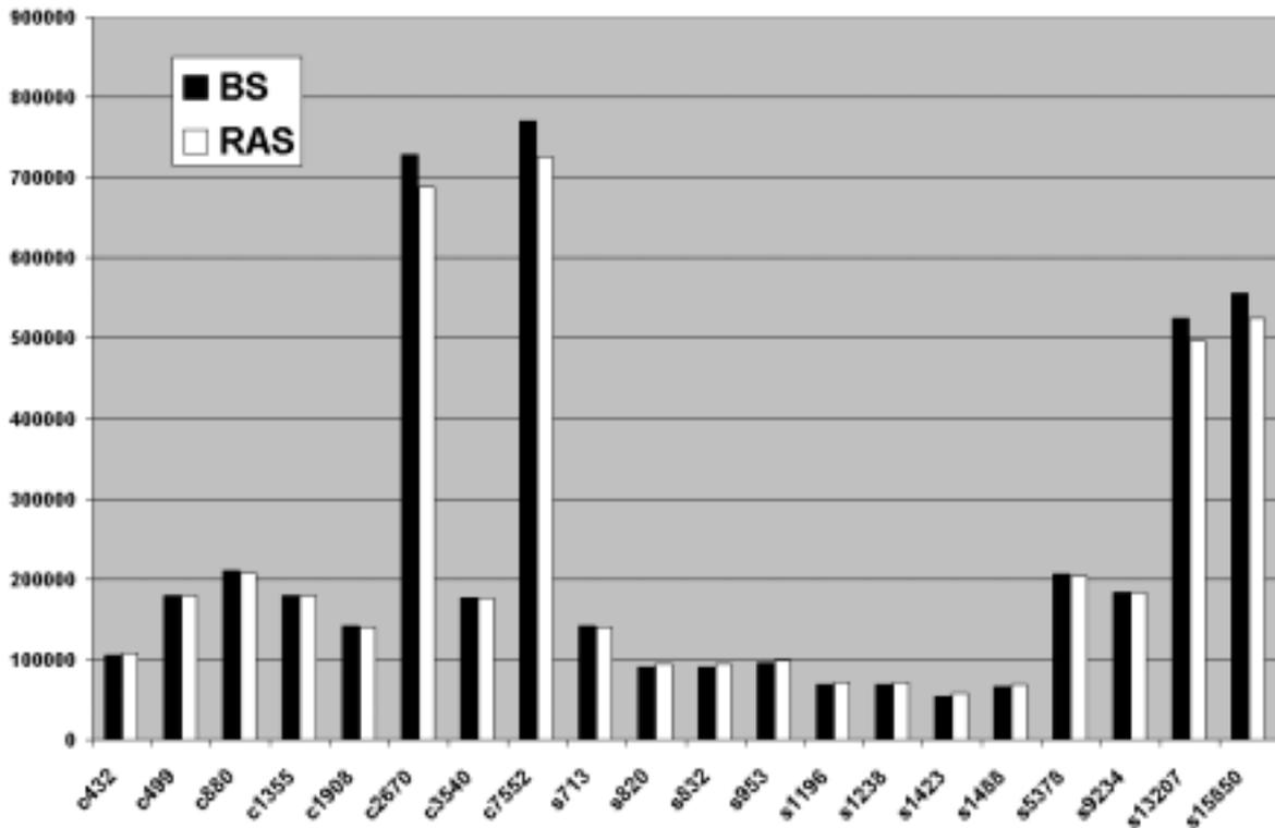
Fig 4: Hardware overhead of the BIST using standard BS compared with the BIST using modified RAS [um<sup>2</sup>] (also Tab. 2).
