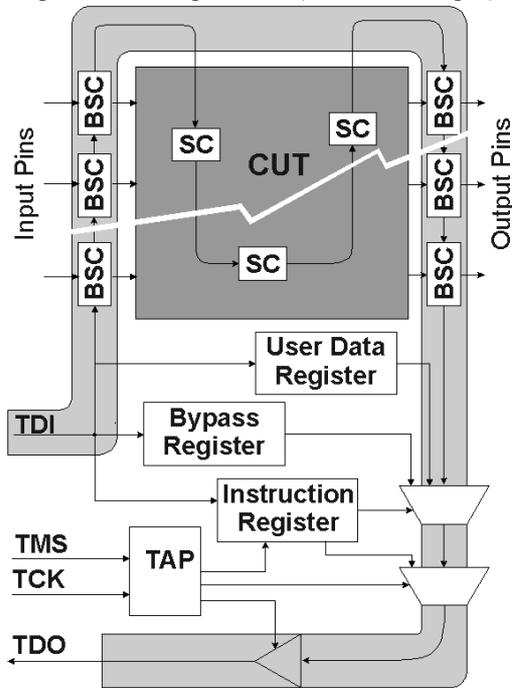
Fig. 1. Boundary Scan on IC
