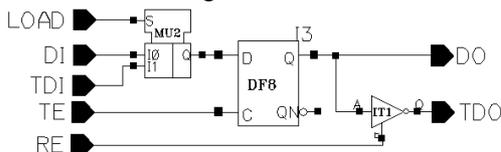
Fig. 4 Reduced I/O cell
