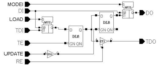
Fig. 5 I/O cell compatible with BS
