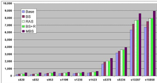
Fig. 3 Hardware overhead (AMS 0.6µm technology Chyba! Nenalezen zdroj odkazů.) of ISCAS circuits using standard BS compared with circuits using modified RAS [thousands of µm²].
